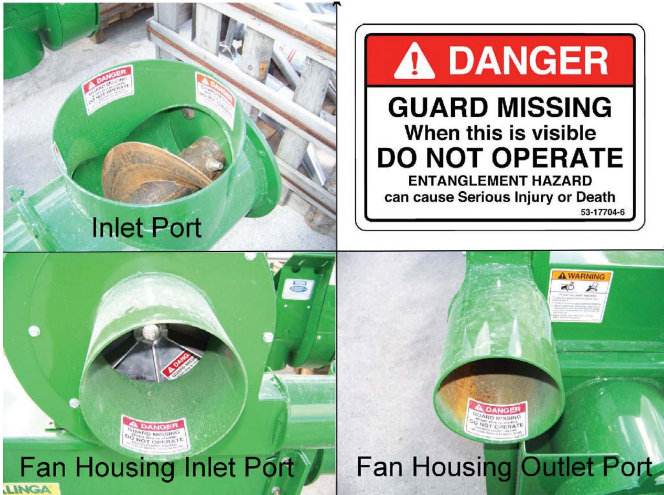
Fig 3-2 SAFETY SIGN: GUARD MISSING
