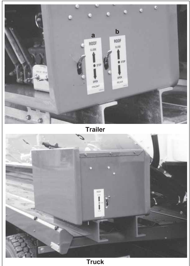
Fig. 4-11 CONTROL BOX (OUTSIDE)
