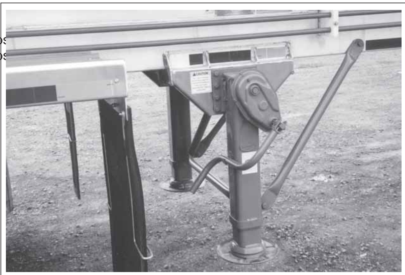
Fig. 6-7 LANDING GEAR MOUNTING BOLTS
