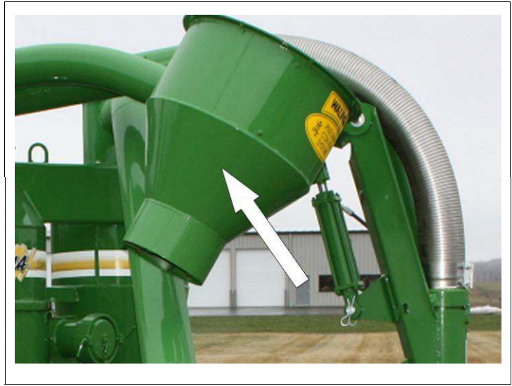
Fig. 5-6 Check the Wearliner in Discharge Cyclone.
