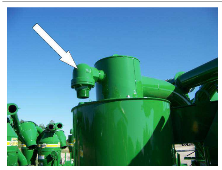
Fig. 5-12 Vacuum Relief Valve.
