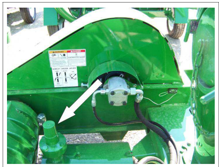
Fig. 5-13 Pressure Relief Valve.
