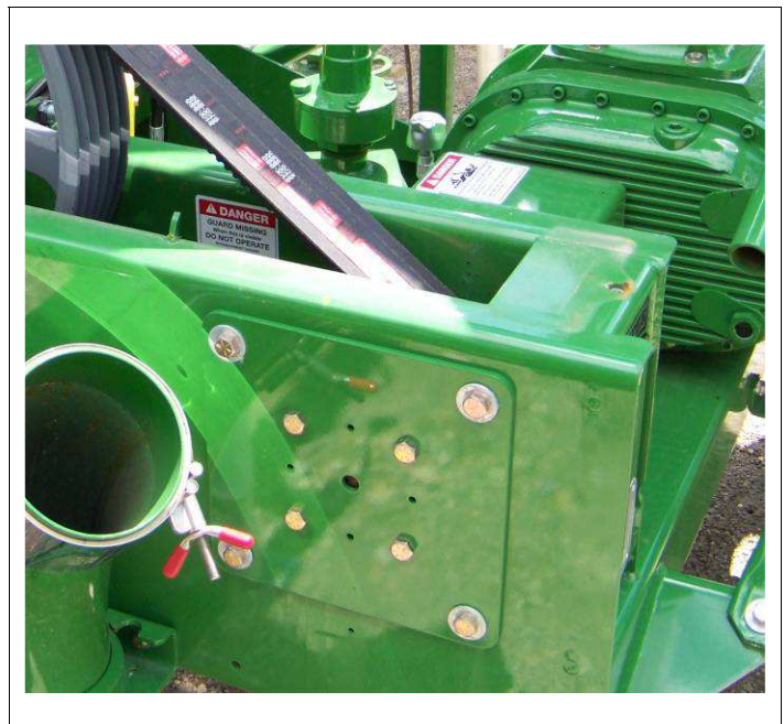
Fig. 5-22 Adjusting Anchor Bolts At Bearing Housing Assembly.
