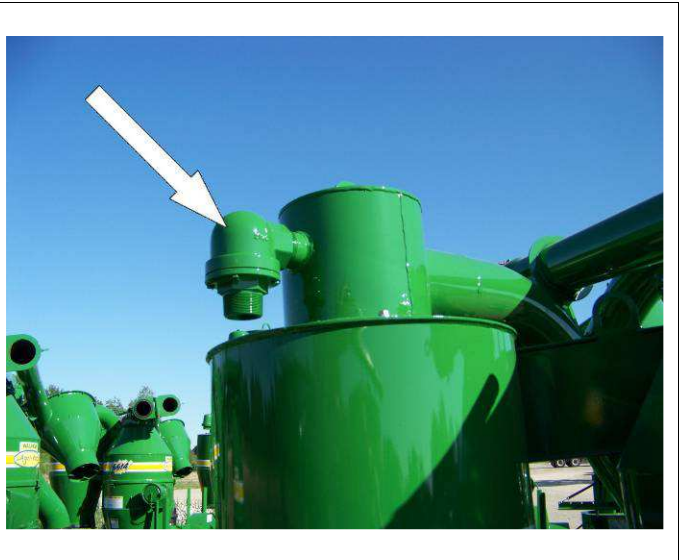
Fig. 5-32 Vacuum Relief Valve.
