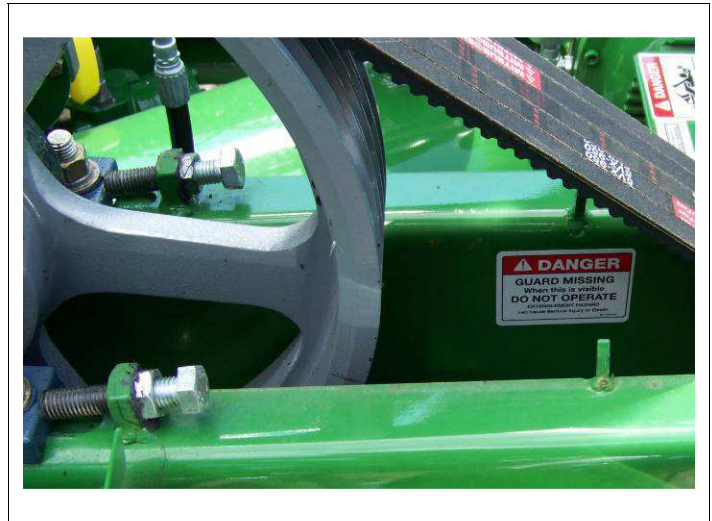
Fig. 5-21 Adjusting Bolts At Input Shaft.
