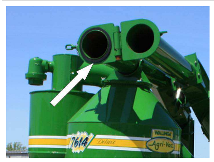
Fig. 5-14 Cyclone Line Seal.
