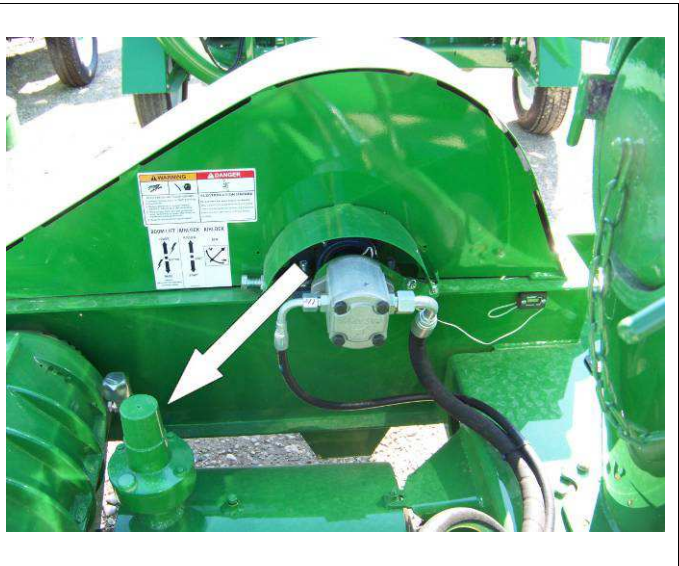
Fig. 5-33 Pressure Relief Valve.
