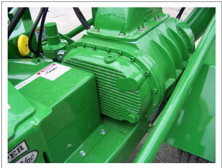
Fig. 5-4 Blower Reservoirs (Front)
