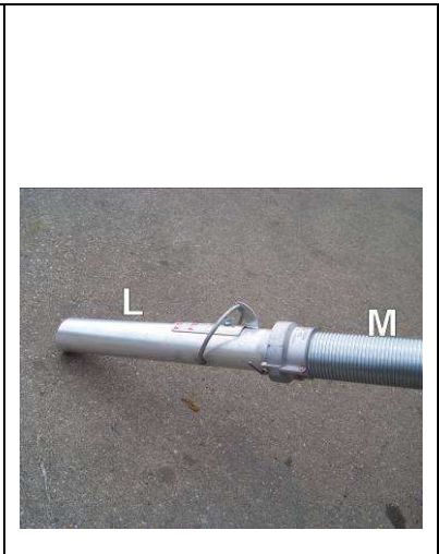
Fig. 4-2 Intake Nozzle & Intake Line
