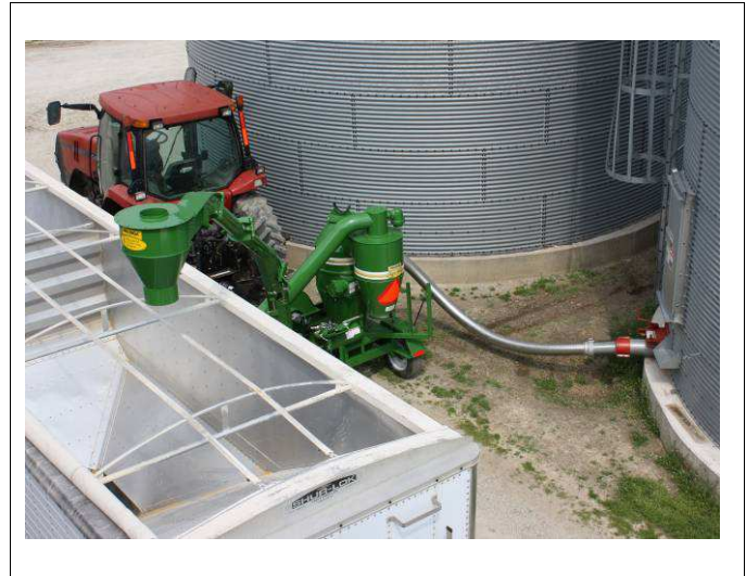
Fig. 4-11 Bin Clearance 12ft (4 M)
