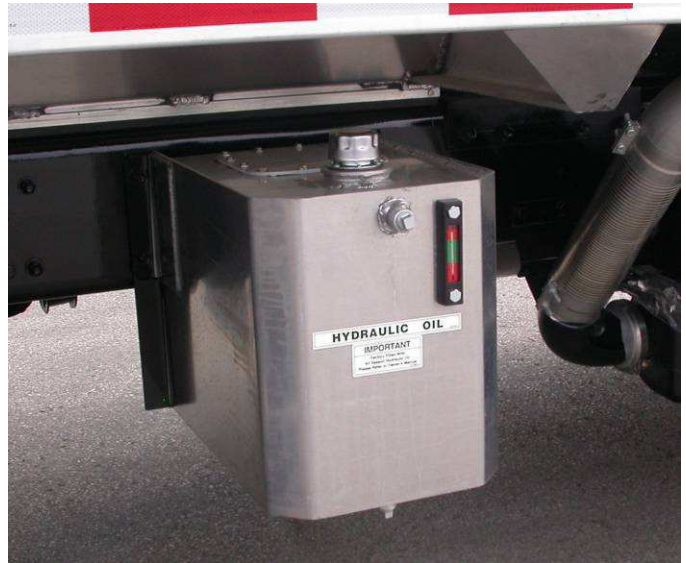
Fig. 7-6 Hydraulic Tank (Typical)
