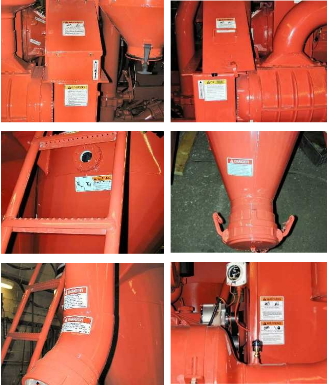
Fig. 3 TYPICAL SAFETY DECALS
